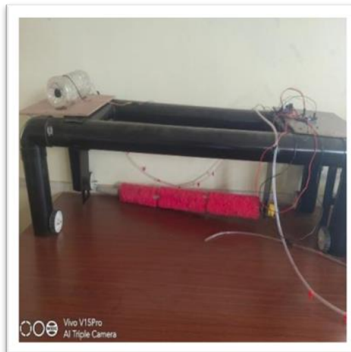
Fig.5.8.3.n Automatic Cleaning Robot for Solar Panel
